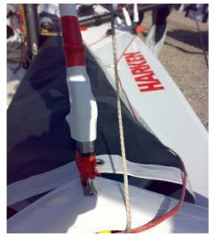
22a. Now tape or cover the chainplate AND the upper eye that the rig tensioning device was attached to, to prevent the spinnaker snagging
