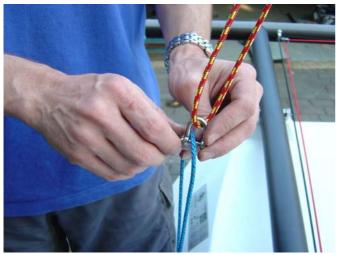
29. You should attach the main halyard to stop it blowing away until you attach it to the mainsail. For your first time, attach it to the outhaul.
