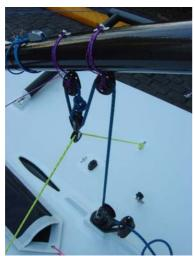
33. Then thread it through the block on the bridal then back through the aft block on the boom and through the jammer. MAKE SURE YOU GET IT THE RIGHT WAY THROUGH
