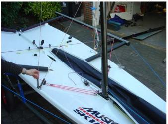
21. Attach the shroud to the outboard rig adjuster. Five holes down on the front row is a good start but check <a href="https://www.mustoskiff.com">www.mustoskiff.com</a> for tuning information
