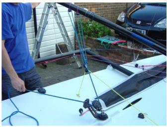
34. Push the boom out to the shroud and cleat the mainsheet.
