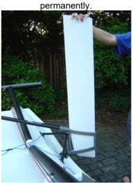
66. Insert the rudder blade. Friction will keep it up.
