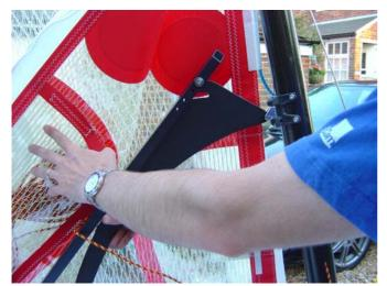
79. Slot the lever and kicker bar together. You may need to apply some leech tension with the mainsheet to achieve this. Make sure the boat is head to wind and if it's windy get some help otherwise the boat can get blown off the trolley.
