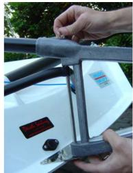
64. Insert the split ring or do up he nut at the top to hold the pin in place. Once on the stock it can be left on the boat
