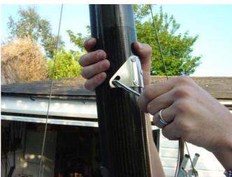
20. With the weight of the mast now on the forestay attach the lower shrouds to the plate on the mast. Do both sides and the mast will now be self supported.
