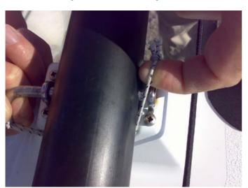
12. Clip the elastic over the pin end between the bar and the deck eye
