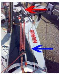
19. Step and hold the mast from blowing sideways. The forestay should be attached loosely with the rig tensioning device (not supplied) to the upper eye (arrowed)
