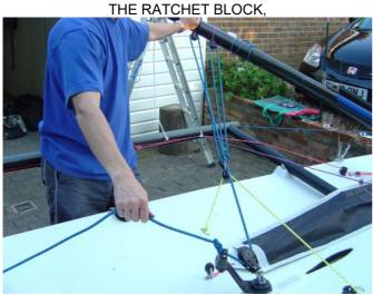
35. Pull the sheet on a little bit and we recommend putting a stopper knot of your choice into the mainsheet; this will stop the boom hitting the shroud when the mainsheet is not cleated.
