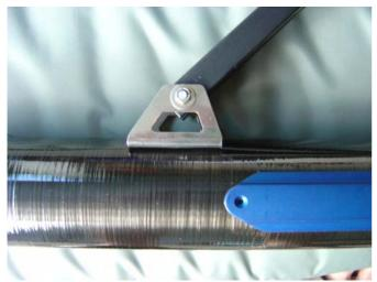
Make sure you don't over tighten this as it will need to move up and down as the kicker is adjusted.
