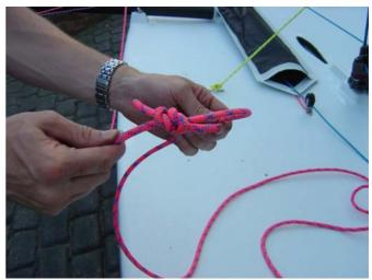
54. Tie or splice the sheet ends together eg using a fishermans knot. Note: For other options- see the pimp section on www,mustoskiff.com.
