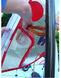
72. Coil the halyard up. It may be placed in the pocket on the side of the main or into some shockcord on spar.
