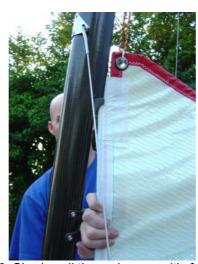
70, Slowly pull the main up, as it's fully battened it can be stiff so go steady. A good spray of suitable lubricant on the <a href="mailto:track can make this easier">track can make this easier</a>.
