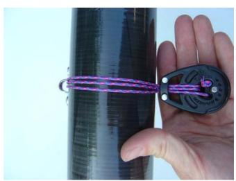
6. Repeat the process until you have several wraps around the boom. Finish the process by tying/splicing the ends off leaving the block "snug" to the boom.
