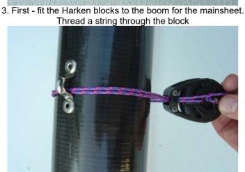
5. Take it through eye on the top of the boom and back through the top of the block. Then back through the body of the block.
