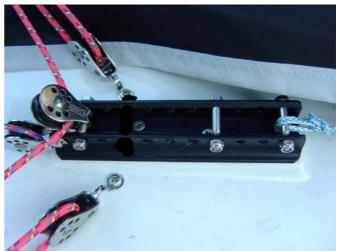
18. Check the mast step is clear to step the mast. The intermediate bolt may be relocated to different holes between the front and back bolts. The back bolt may be moved to the back holes. The kicker control line & vang rope block may be relocated to another part of the step.
