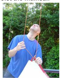
69. Check the halyard doesn't have any twists and shackle the head on.
