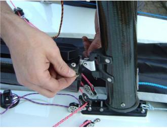
28. Remove the pin in the lower gooseneck and fit it through the boom.
