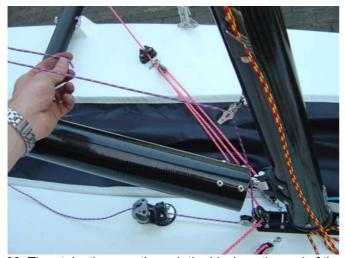
39. Then take the rope through the block on the end of the lever and back towards the mast.
