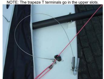
17. Attach the lower shroud to the inboard rig adjuster. Five holes down on the front row is a good start but check <a href="https://www.mustoskiff.com">www.mustoskiff.com</a> for tuning information
