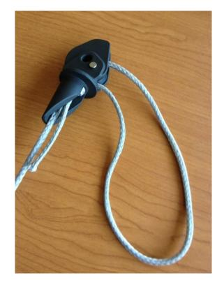
4. Regular maintenance is a must-Movement of the knot to avoid halyard chafe helps avoid breakage
