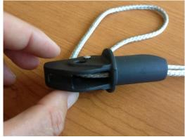
2. Loop over the line and feed back through the casting and down the mast via a mouse-line.
