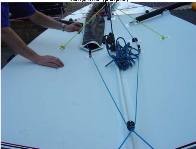
45. Through the "take up" block at the back of the boat and through the block at the back of the chute.
