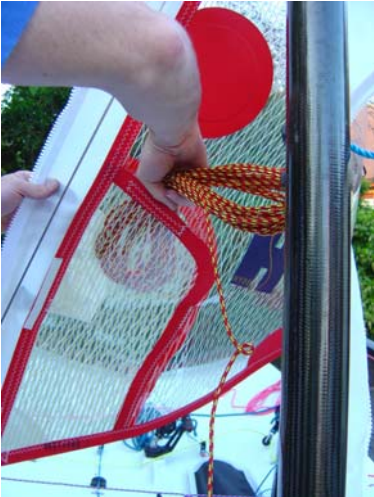
72. Coil the halyard up. It may be placed in the pocket on the side of the main or into some shockcord on spar.
