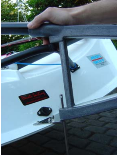
63. Offer the stock up to the pintles and insert the pin from below the bottom pintle plate
