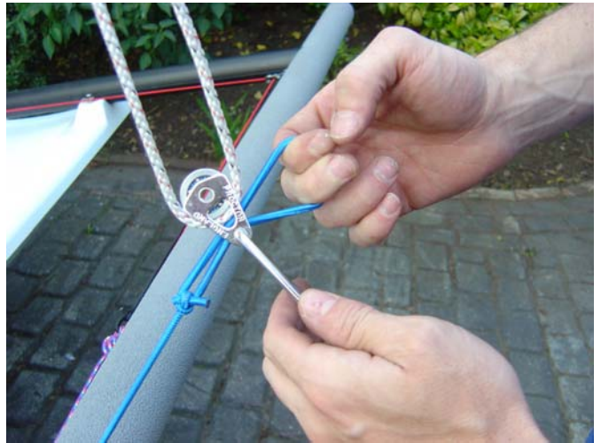
24. Take the loop and pull it through the ring block.
