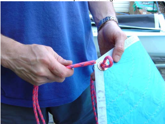
51. Then you may attach the kite sheets to the clew. There are various options for attaching the sheets, some are shown on the class website, The method shown involves finding the middle of the sheets and push the loop through
