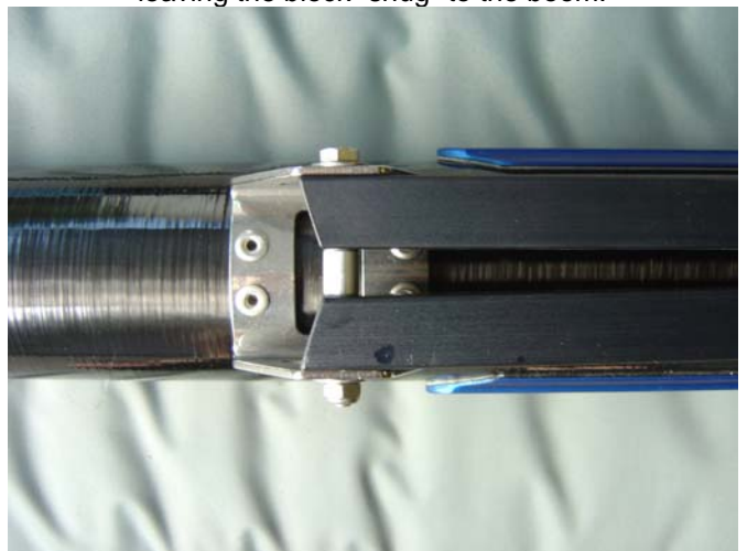
8. Bolt the double kicker bar to the boom fitting
