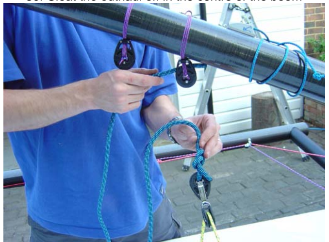
32. Rig the mainsheet starting with a knot at the block attached to the mainsheet bridal. The method of tying is optional. Then thread it through the front block on the boom.
