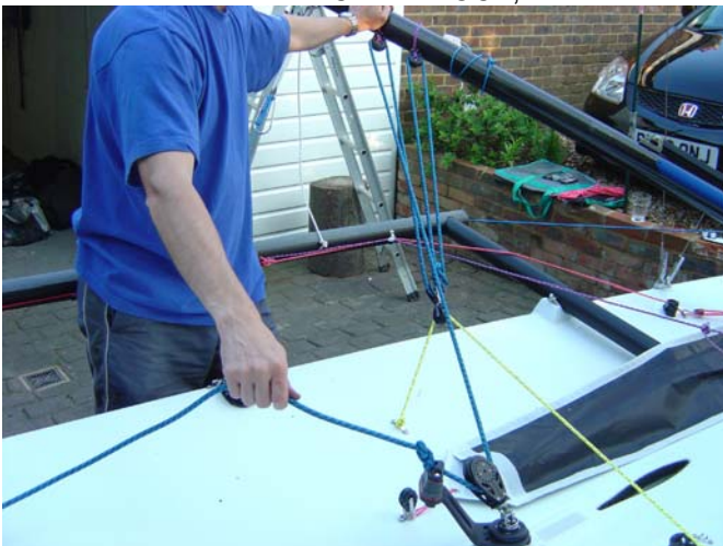
35. Pull the sheet on a little bit and we recommend putting a stopper knot of your choice into the mainsheet; this will stop the boom hitting the shroud when the mainsheet is not cleated.
