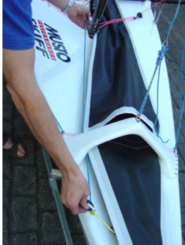
41. Take the halyard from the exit on the front of the mast, under the chute throat and through the block attached to the pole "puller"
