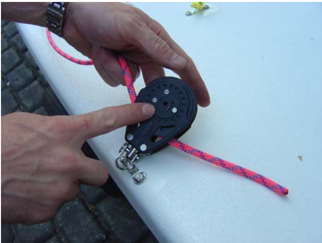
53. Thread the sheet ends through the ratchet blocks, observing the arrow on the blocks to make sure that the ratchet is working in the correct direction
