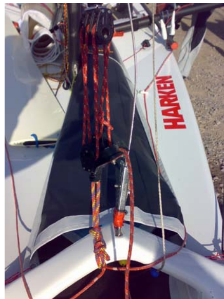
22. Now you have both shrouds and lowers are attached tension the rig using the tensioning device and then locate the lower eye (shown blue arrow in step 19) into the chainplate and insert the pin. Then remove the tensioning device. NOTE: Please don't over tension the rigging; call Ovington Boats if unsure on required rig tension.
