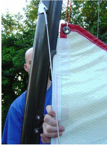
70. Slowly pull the main up, as it's fully battened it can be stiff so go steady. A good spray of suitable lubricant on the track can make this easier.
