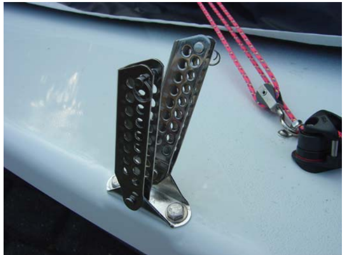
16. Fit the rig adjusters onto the chain plates
