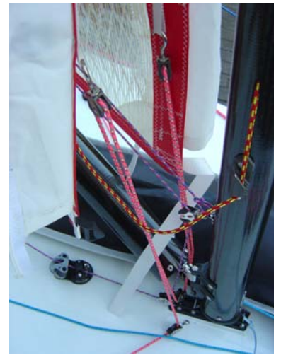
83. Make sure there are no twists in the system and everything is the correct side of boom and not twsited.
