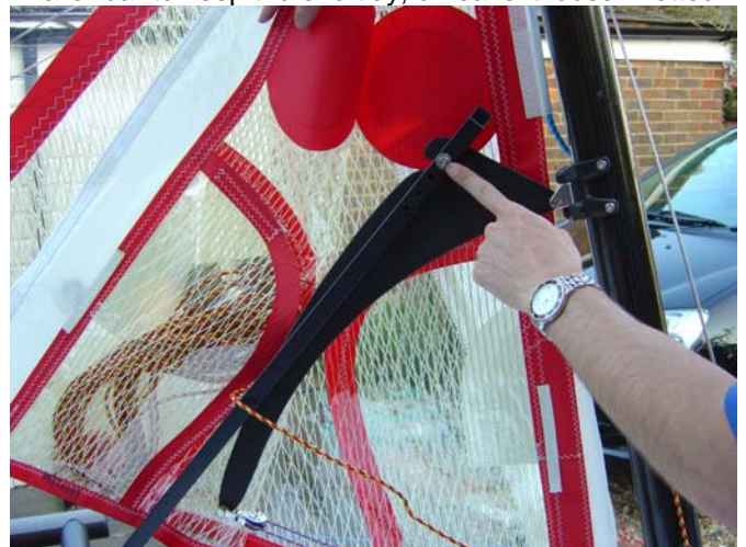
80. The bolt should be in the top of the four available holes.
