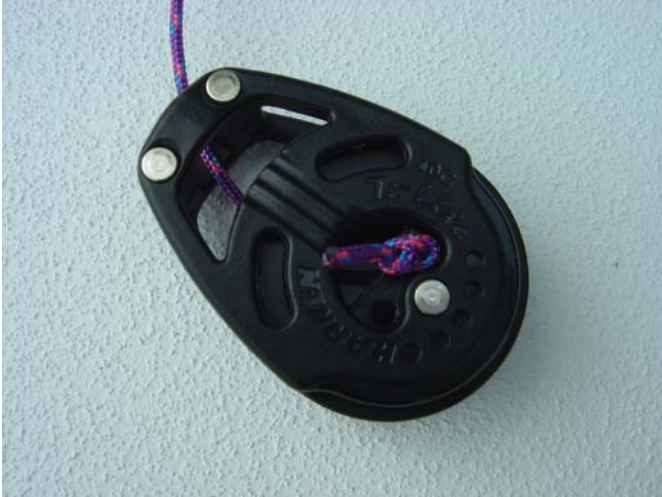
3. The first step is to fit the Harken blocks to the boom for the mainsheet. Thread a string through the block
