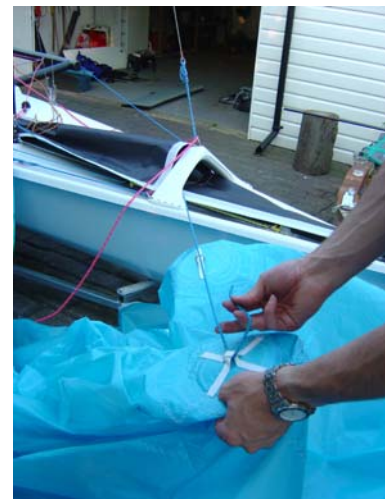
58. Tie the downhaul to the upper patch on the kite.
