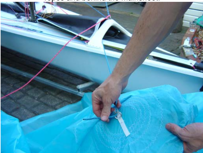
57. Un-tie the downhaul from the forestay eye (remember step 49) thread it through the ring on the kite. Make sure you are under the kite sheets
