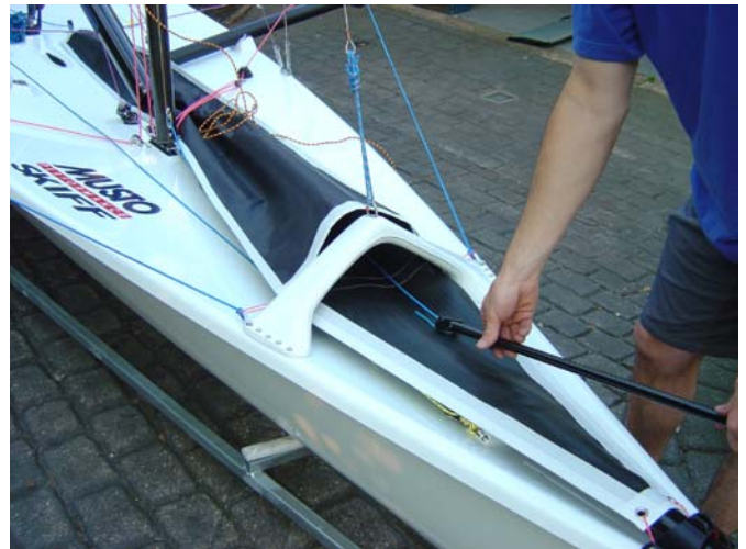
48. Pull the extension out of the chute
