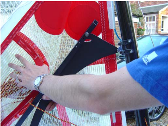
79. Slot the kicker bars together. You may need to apply some leech tension with the mainsheet to achieve this. Make sure the boat is head to wind and if it's windy get some help otherwise the boat can get blown off the trolley.
