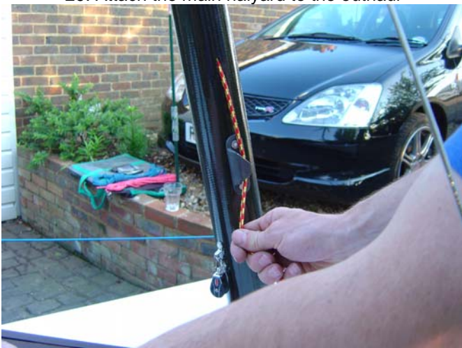
31. Pull some of the main halyard through so the boom is in the approximate position that you would expect when sailing
