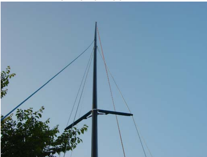
61. Have a quick look up to make sure the halyard is not twisted or inside a shroud.
