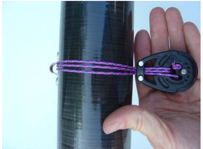
6. Repeat the process until you have several wraps around the boom. Finish the process by tying/splicing the ends off leaving the block "snug" to the boom.
