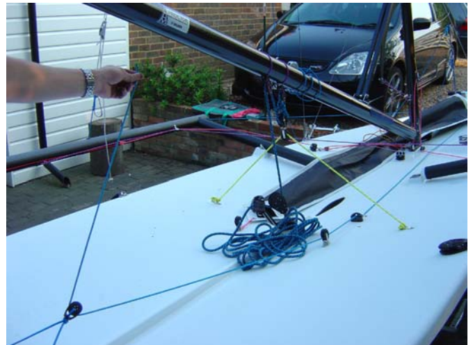
44. Through the cleat on the deck and through the block behind it. Note: Make sure you go under the bridle.
