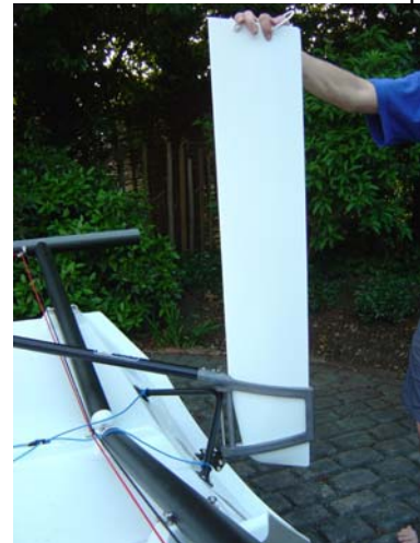
66. Insert the rudder blade. Friction will keep it up.
