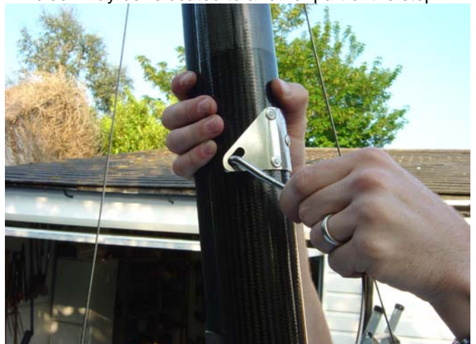
20. With the weight of the mast now on the forestay attach the lower shrouds to the plate on the mast. Do both sides and the mast will now be self supported.
