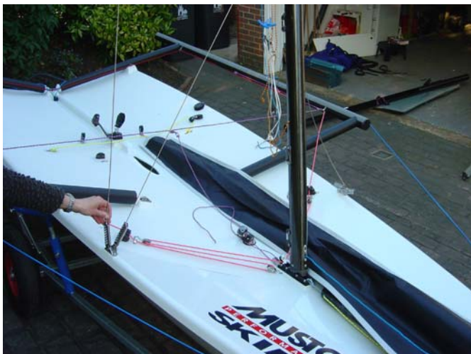
21. Attach the shroud to the outboard rig adjuster. Five holes down on the front row is a good start but check www.mustoskiff.com for tuning information
