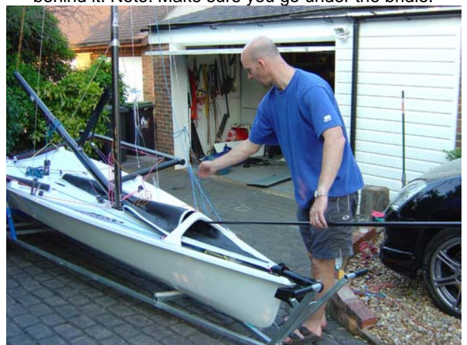
46. Use the tiller extension to thread the halyard through the chute.
