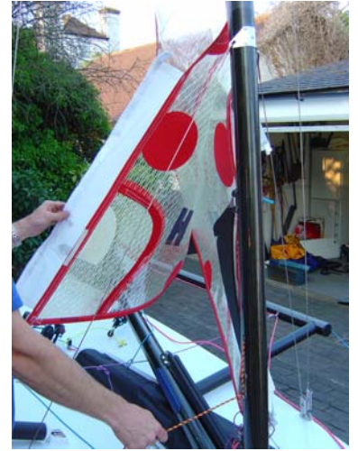
71. Once it is at the very top give the halyard a good pull and cleat it off.
