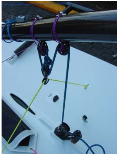
33. Then thread it through the block on the bridal then back through the aft block on the boom and through the jammer. MAKE SURE YOU GET IT THE RIGHT WAY THROUGH THE RATCHET BLOCK,
