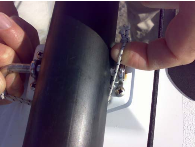
12. Clip the elastic over the pin end between the bar and the deck eye
