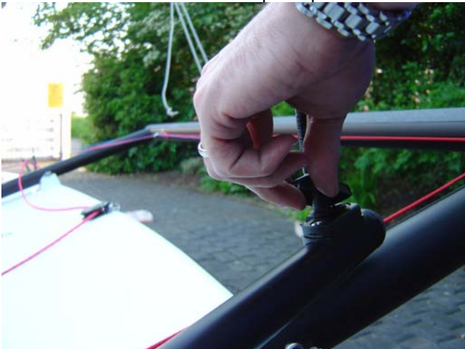
65. Clip the tiller extension onto the tiller.
