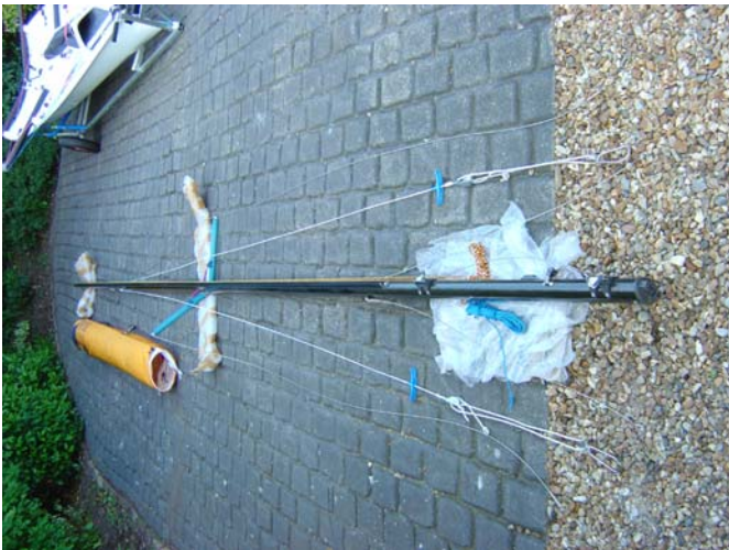
15. Before stepping the mast lay it out (on padding, you don't want to scratch your new carbon mast). Check the lines and wires are not twisted up. LOOK UP to check you are not going to hit anything when you raise mast, especially power lines!! NOTE: The trapeze T terminals go in the upper slots.
