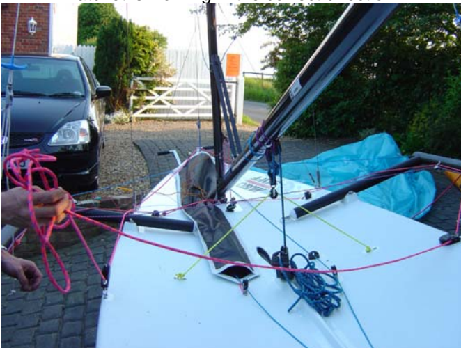
55. Make sure you have run the kite sheets on top of other ropes and behind the mainsheet.
