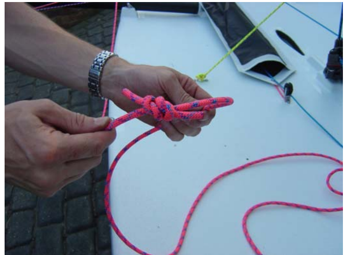
54. Tie the sheet ends together using a fishermans knot. Note: You can tie the sheet ends to the clew if you want but I prefer this method. There are also other options for this.
