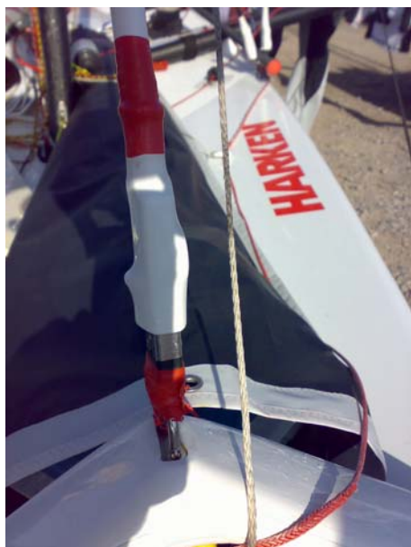
22a. Now tape or cover the chainplate AND the upper eye that the rig tensioning device was attached to prevent the spinnaker snagging
