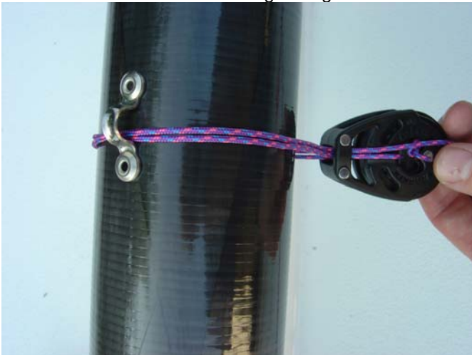
5. Take it through eye on the top of the boom and back through the top of the block. Then back through the body of the block.
