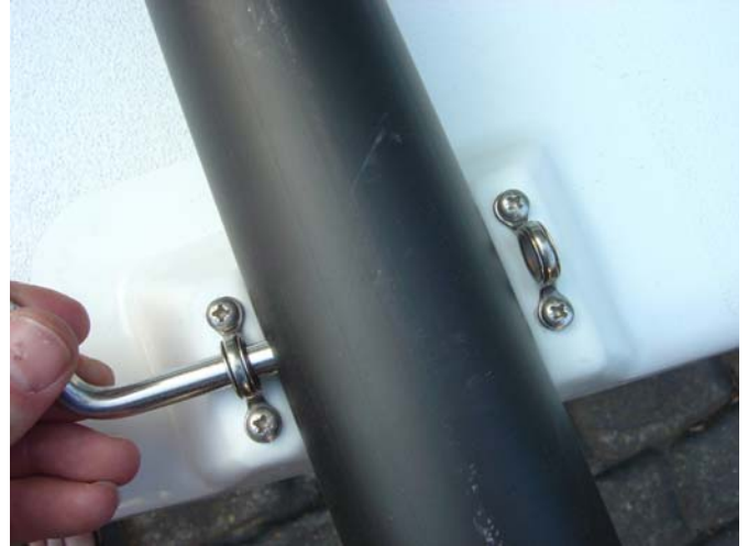
11. Insert the wing pins. If they are difficult to insert you may not have the wings in properly. Give them a little "wiggle" until the pin can be inserted.
