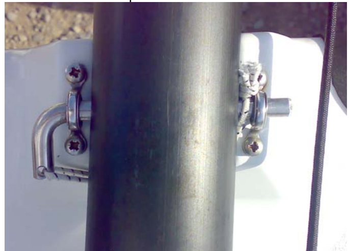
13. With the elastic between the wing and the deck eye the elastic can never get knocked off and you won't lose any pins. The folded ends of the pins should preferably be away from the cockpit so that ropes don't get caught on the pin.
