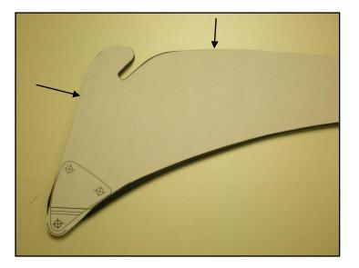
Cut off the material below the line marked on the template and drill the two marked holes out to 5.5mm – use a centre punch to accurately locate your holes.
